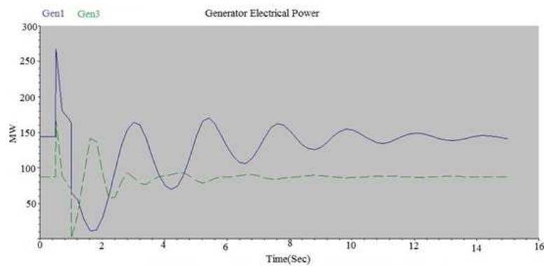
Figure 11: Generator Electrical Power with PSS and Shunt Capacitor
