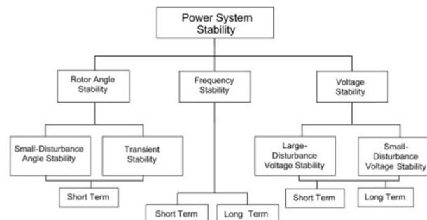
Figure 1: Classification of Power System Stability
