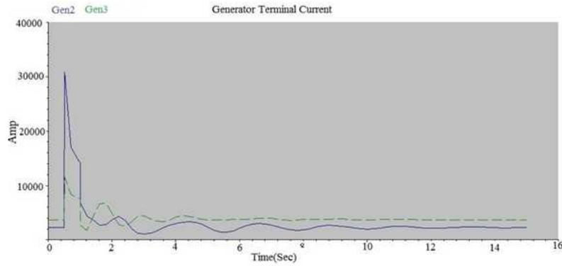
Figure 8: Generator Terminal Current without PSS and Shunt Capacitor
