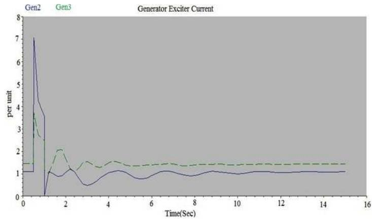
Figure 6: Generator Exciter Current without PSS and Shunt Capacitor
