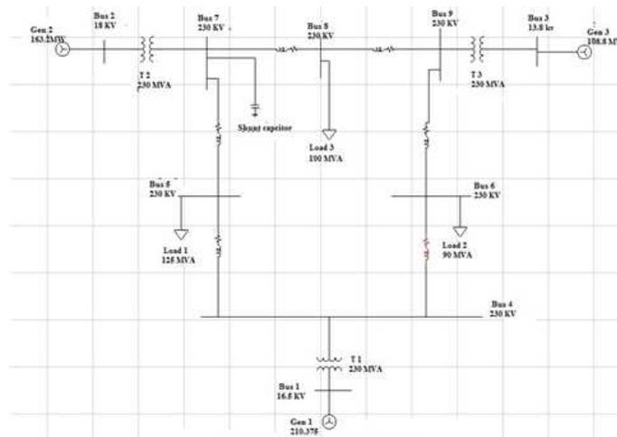
Figure 3: 9 Bus Multi-Machine System
