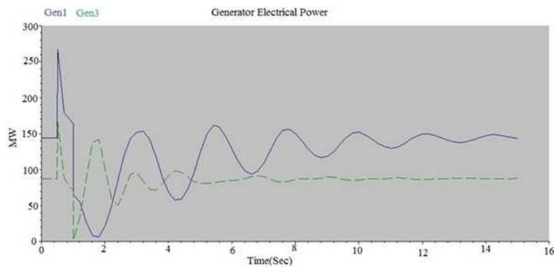
Figure 10: Generator Electrical Power without PSS and Shunt Capacitor
