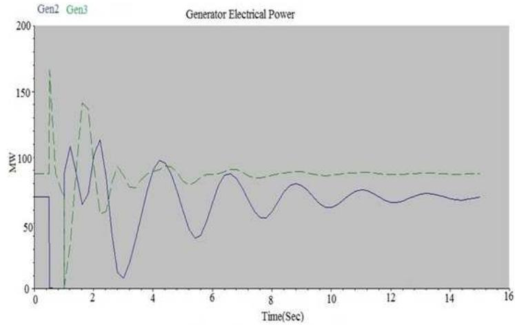
Figure 5: Generator Electrical Power with PSS and Shunt Capacitor
