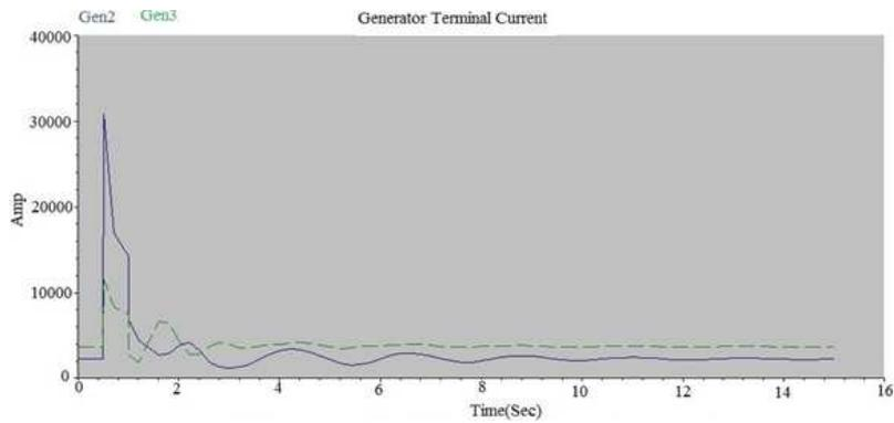
Figure 9: Generator Terminal Current with PSS and Shunt Capacitor
