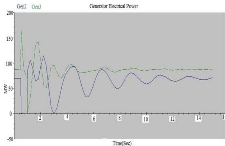
**Figure 4: Generator Electrical Power without PSS and Shunt Capacitor**
