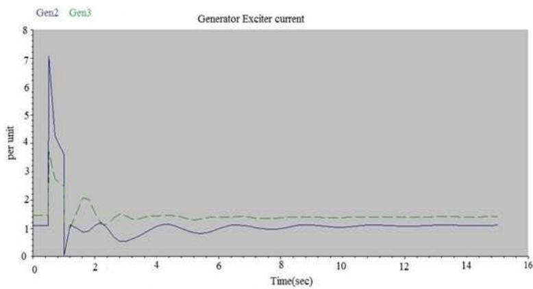
Figure 7: Generator Exciter Current with PSS and Shunt Capacitor
